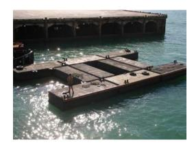
The units join together with 4 sets of ISO freight container twist locks and castings.
